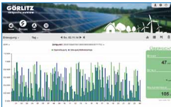
Energy balance of a plant in accordance with German law (EEG) compared with a reference plant
